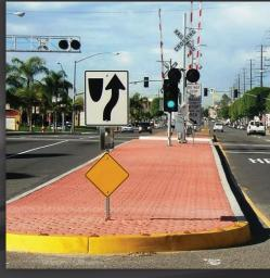
Additional crossing gate arms to deter motorists from crossing the tracks when a train is passing
